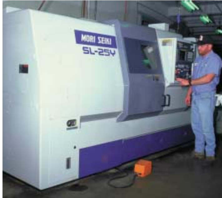
Diameter x 42" Long. Turret is Equipped with "Y" Axis and Live Tooling. Machine is Equipped with Steady Rest, P/Tail Stock and Chip Conveyor
