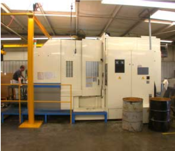
Okuma M50H Horizontal Milling Center - 40 Tools, 24" x 31" Pallet
